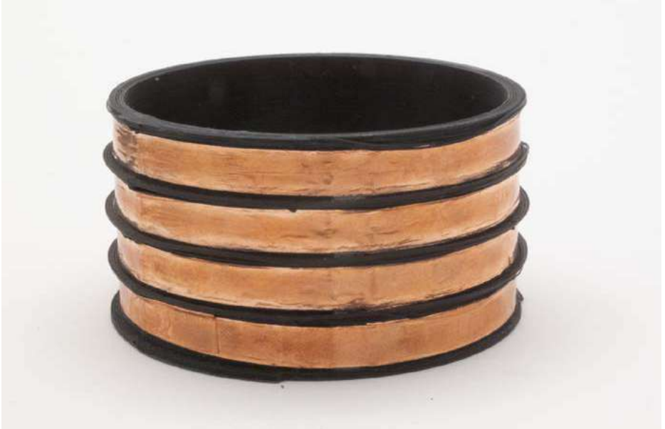
Figure 17: Slip ring, showing copper tape around circumference
