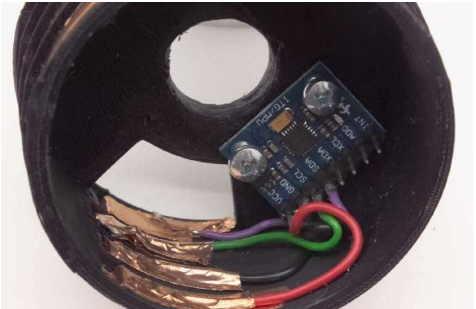
Figure 18: Slip ring, showing inside connections
