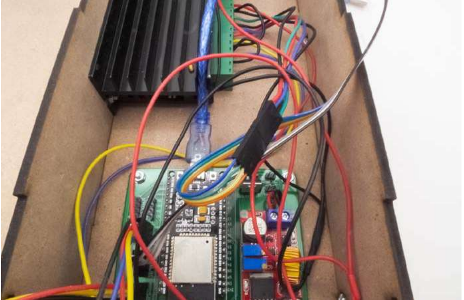
Figure 29: Microstepping control board wiring
