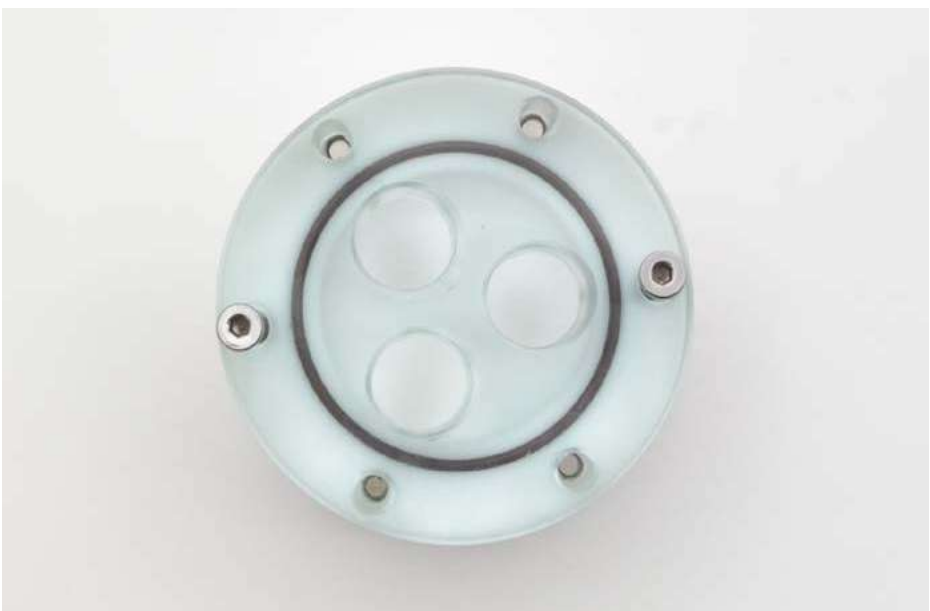
Figure 16: Vessel with glass top, partially screwed together
