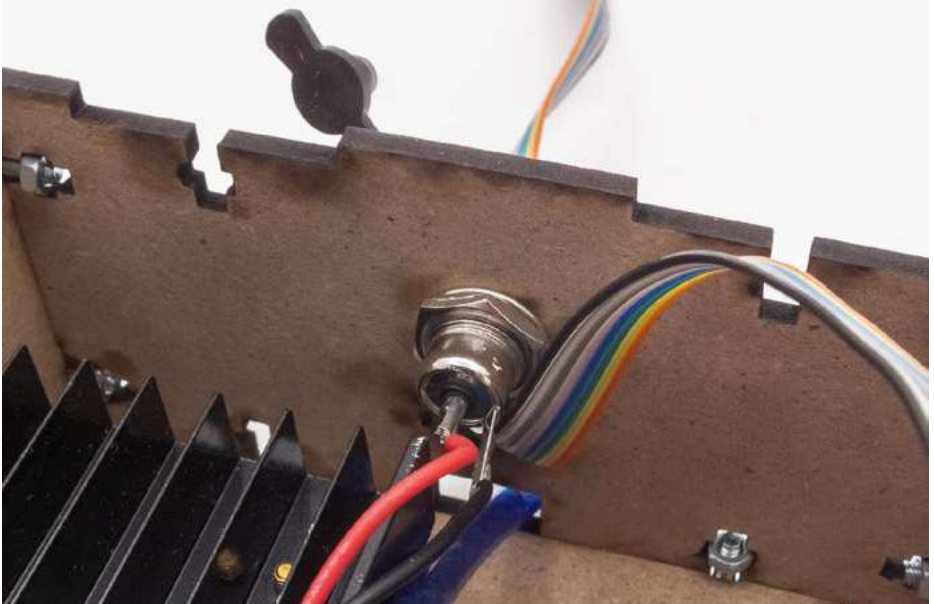
Figure 28: 5.5x2.1mm plug wiring
